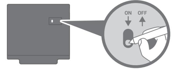
Start of operation: Use a pen to push the switches on the back of the CSI Board downwards. Switch off again when not in use.
