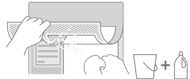
If the adhesive properties diminish with time or if the display becomes soiled clean the adhesive seal and suction pads using a mild detergent (not a window cleaner).
