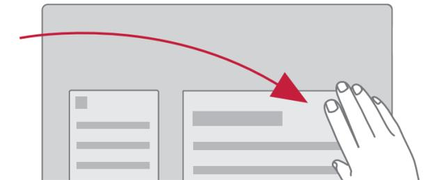
Close the foil cover, making sure the edges are pressed down well in particular, so that the display is sealed properly on all sides.
