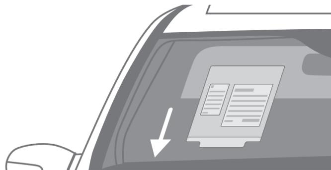
Insert the CSI Board on the inside of the windscreen (stop at resistance, otherwise the vehicle might get damaged) and position it correctly.
